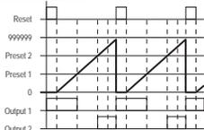
The display continues to increase/decrease until the overflow or underflow value is reached. Output 1 is held while the present value is less than or equal to Preset 1. Output 2 is held while the present value is greater than or equal to Preset 2.
