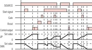
Timing starts when the start signal goes ON. \*Note1 The control output is controlled using a sustained or one-shot time period.
