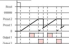
Present value display does not change during 1-shot time period, but reset start status is returned to as soon as count is reached. Outputs are 1-shot and operate repeatedly. Output 1 is self-holding, and goes off after expiration of the 1-shot period for Output 2. One-shot time periods for Output 1 and 2 are independent.
