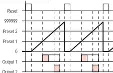
Present value runs continuously. Output 1 is self-holding, and goes off after expiration of the 1-shot period for Output 2. One-shot time periods for Output 1 and 2 are independent.
