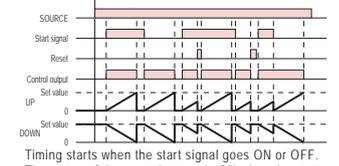
Timing starts when the start signal goes ON or OFF. The status of the control output is ON when the start signal goes ON or OFF.
