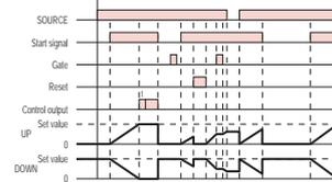
Timing starts when the start signal goes ON, and is reset when the start signal goes OFF. \*Note1 The control output is controlled using a sustained or one-shot time period.
