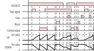
Timing starts when the start signal goes ON. \*Note1 The status of the control output is reversed when time is up (OFF at start).
