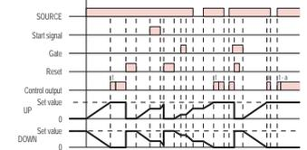
Timing starts when the reset input goes OFF. The start signal disables the timing function (i.e., same function as the gate input). The control output is controlled using a sustained or one-shot time period.
