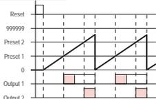
Present value runs continuously through 1-shot time period and returns to reset start status immediately afterward. Outputs are 1-shot and operate repeatedly. Output 1 is self-holding, and goes off after expiration of the 1-shot period for Output 2. One-shot time periods for Output 1 and 2 are independent.
