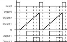
The display continues to increase/decrease until the overflow or underflow value is reached. Output 1 is held while the present value is greater than or equal to Preset 1. Output 2 is held while the present value is greater than or equal to Preset 2.
