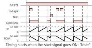
Timing starts when the start signal goes ON. \*Note1 The status of the control output is reversed when time is up (OFF at start).
