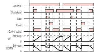
Timing starts when the start signal comes ON. \*Note1 The control output is reset when time is up.
