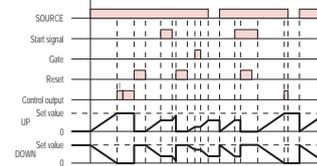
Timing starts when the reset input goes OFF. The start signal disables the timing function (i.e., same function as the gate input). The control output is controlled using a sustained or one-shot time period.
