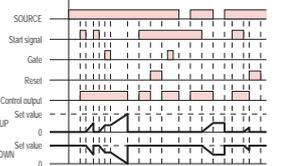
The control output is ON when the start signal is ON (except when the power is OFF or the reset is ON). The timer is reset when the time is up.
