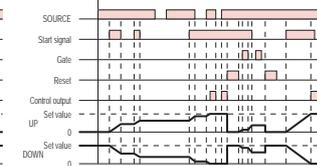
Start signal enables timing (timing is stopped when the start signal is OFF or when the power is OFF). A sustained control output is used.
